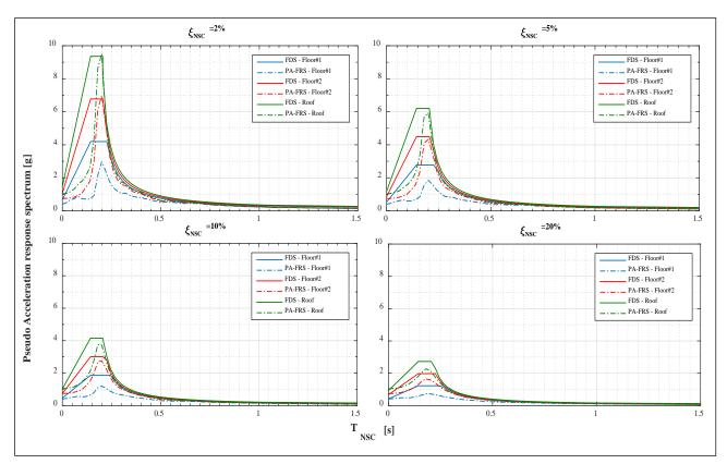
Figure 2 – Comparison of the proposed FDS and the PA-FRS generated for all floors of Building#4 considering NSCs damping ratios of 2, 5, 10, and 20 %
