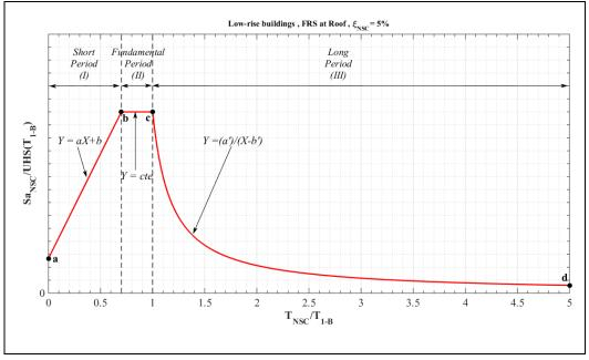
Figure 1 – Schematic of the proposed FDS and idealization of spectral acceleration for NSCs
