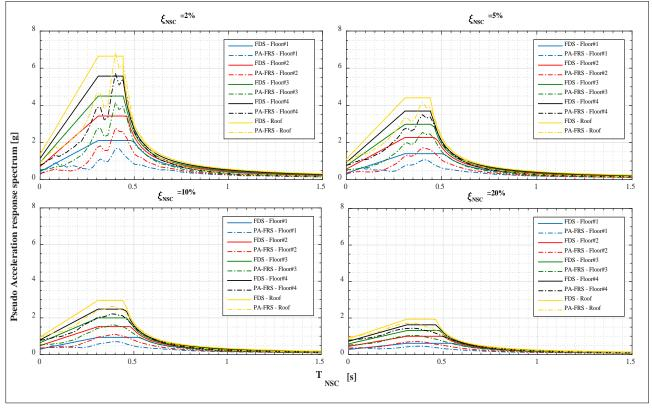
Figure 3 – Comparison of the proposed FDS and the PA-FRS generated for all floors of Building#18 considering NSCs damping ratios of 2, 5, 10, and 20 %
